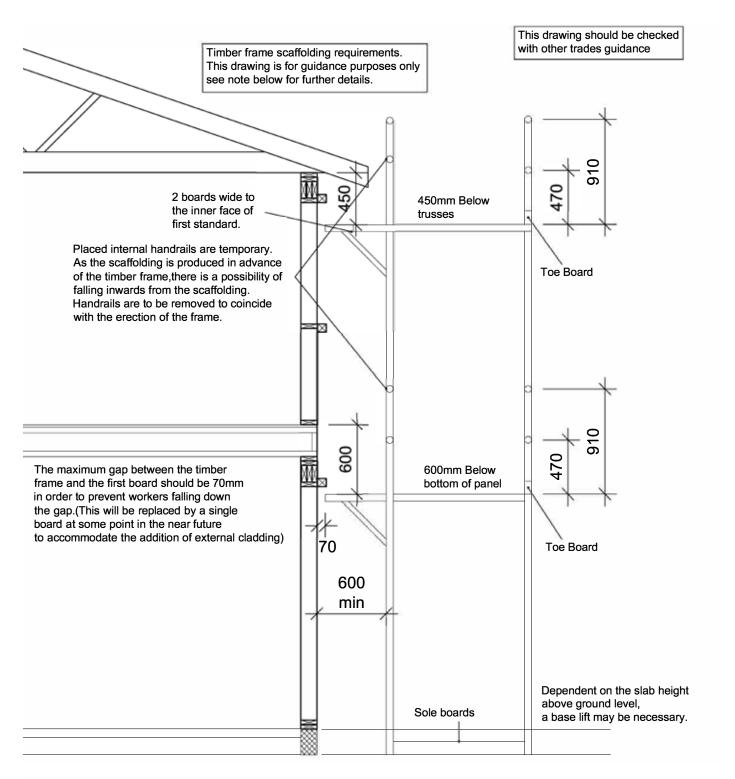
Note: Freestanding scaffold that cannot be tied into timber frame. This must be structurally designed in accordance with British standard EN121811-1 and NASC TG20:05. Consideration must be given to the provision of takers, outriggers, guys, etc to stabilise the scaffold. The perimeter scaffold most be fully erected prior to the standing of the timber frame.
