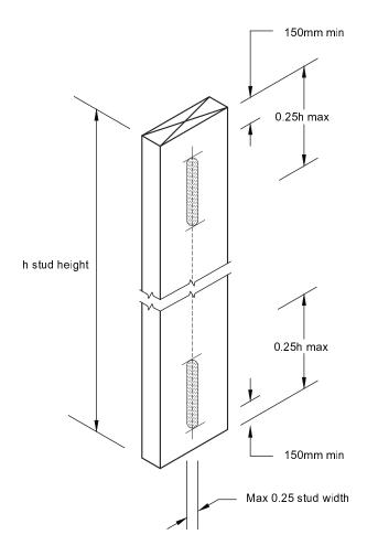
Stud frames should not normally be notched. When this is unavoidable then notches should be as small as possible and positioned towards the end of a stud.
