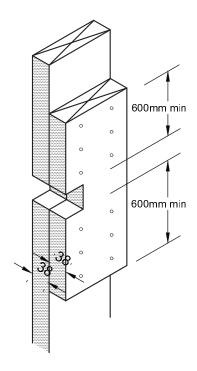
Heavily loaded studs should be reinforced as shown.
